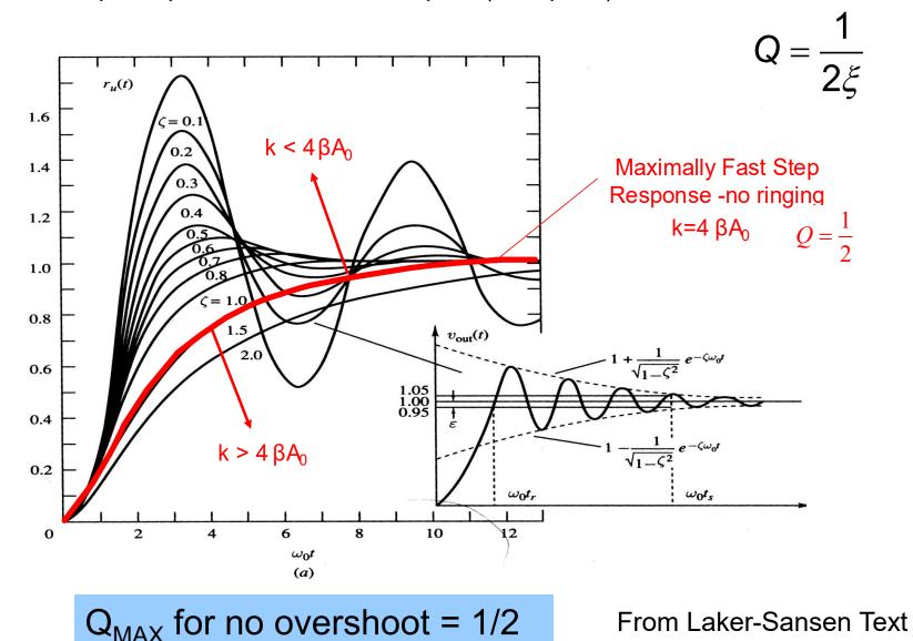
For two-stage amplifiers, must have open-loop pole spread, k, very large to avoid ringing in step response
