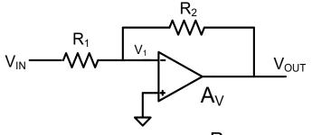
$$A_{VF} = \frac{V_{OUT}}{V_{IN}} = \frac{-\frac{R_2}{R_1}}{1 + \frac{1}{A_V} \left(1 + \frac{R_2}{R_1}\right)}$$
