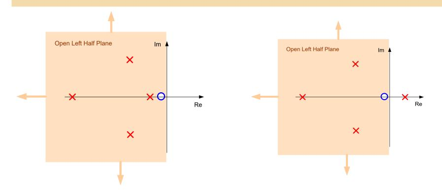
Stable with two negative real axis poles, two LHP complex conjugate poles, and two LHP CC poles
